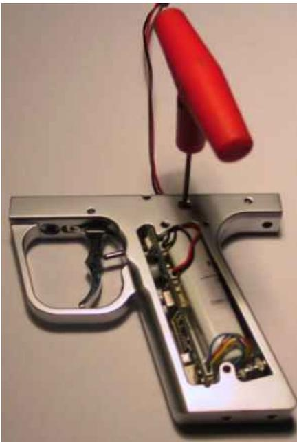
Check if there is room for the spacer on the right side of the solenoid by trying to slide it in.
