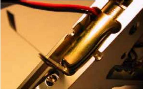
Adjust the FreeKICK spacer in front of the solenoid so that the sear actuator is just touching the solenoid pin (you might want to use some smaller pliers than me).
