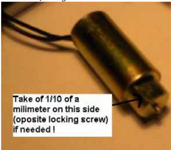
Make sure that you get all the metal dust of the solenoid before reinstalling it in the grip.
