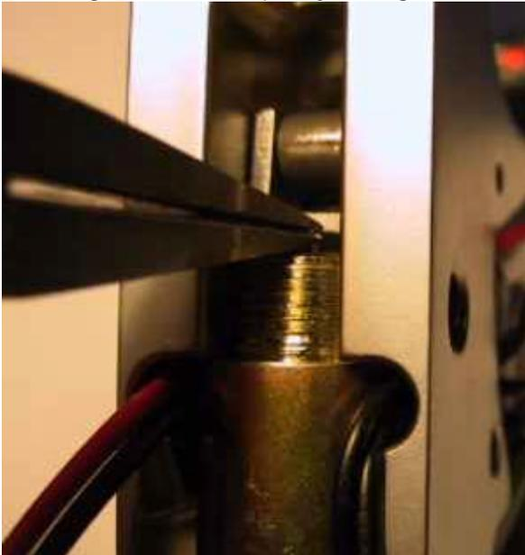
Then tighten the solenoid lock screw (don't overdo it - just snug it up and then a slight nudge) making sure nothing moves around.
