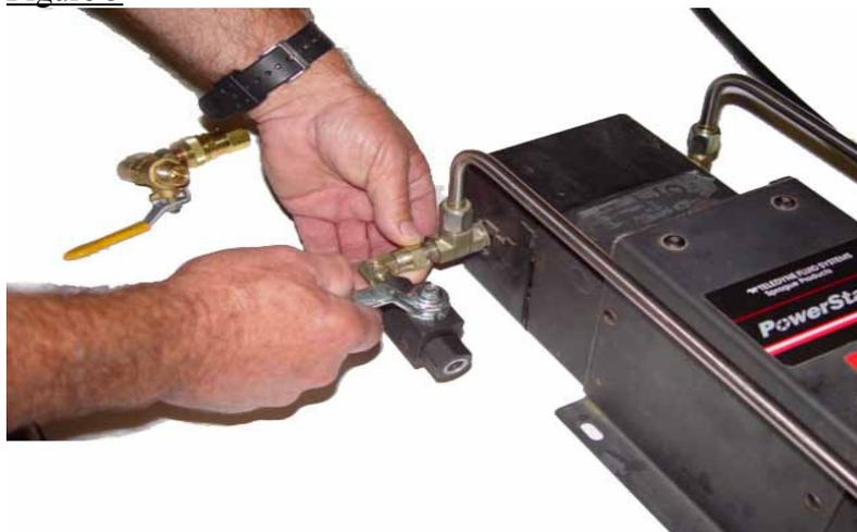
Step 2. After securing the Megabooster, next install the inlet side air valve. Do this by attaching the compression fitting to the inlet side of the Megabooster. To properly orient the Megabooster, see Figure 3. Note that the small red plug where the drive air assembly attaches is close to you when the system is ready for use. Once attached, tighten the compression nut to 20 ft/lbs (Figure 5)
