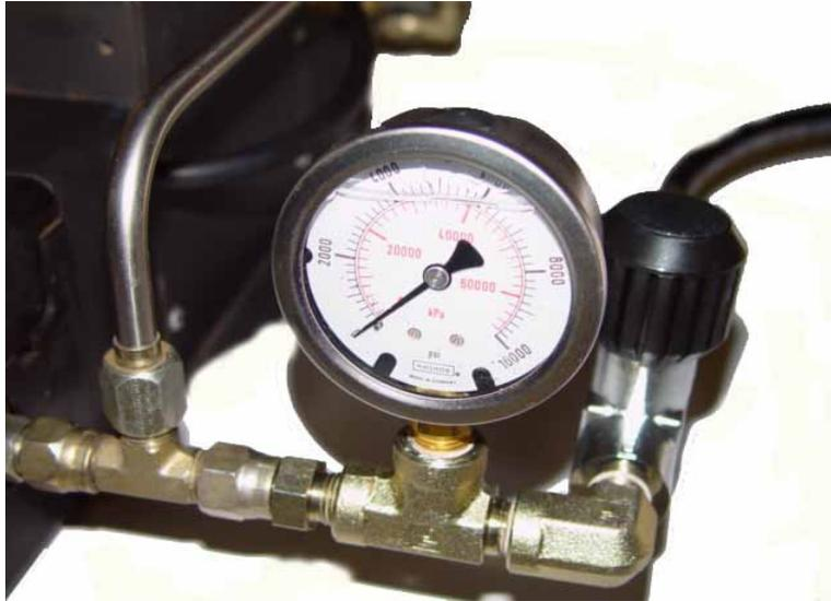
Step 6. Slowly open the fill lever (Figure 14) to allow pressure from the paintball cylinder to equalize the pressure in the fill line from the Megabooster to the paintball cylinder. At this stage note the pressure on the Megabooster gauge. DO NOT pay attention to the gauge on the paintball tank, the Megabooster gauge is much more accurate.
