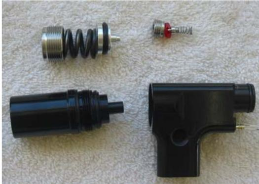
pin to allow air to escape between the pin and seal. The pressure of the escaping air pushes back against that piston, compressing a spring until the piston no longer presses against the pin and air is sealed. Correct pressure. Air is used, pressure drops, pressure against springs is reduced, spring expands pushing piston, piston pushes pin allowing air to escape. Screw down the cap for higher pressure. Unscrew the cap for lower pressure. Perfect!
