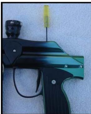
NOTE: the two adjustment screws are opposite. Screwing clockwise increases the travel on one, but decreases travel on the other. Make small adjustments until you are sure which way you need to turn. Half turns are adequate. Large movements mean you are turning the wrong way.
