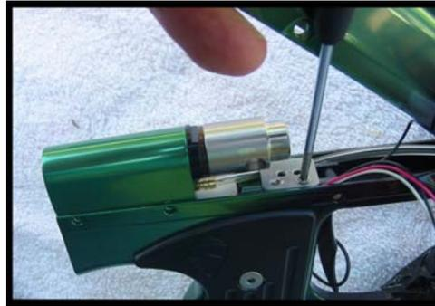
Remove the trigger spring in the trigger. Additionally note that the eye wires go
