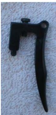
Back setscrew hits ledge in trigger frame. Front cap screw hits plate.
