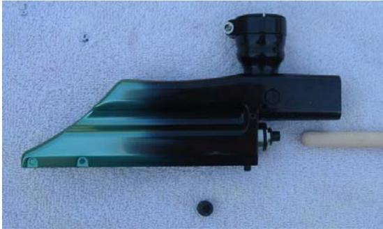
First, put the pin in the valve. While pushing on the valve pin and carefully aligning the valve body so that the O-Rings are not cut, slide the valve into the body making sure the hole is at the top and the alignment recess for the setscrew is at the bottom. Setscrew the valve in place once valve properly centered. Place the spring on the valve pin.
