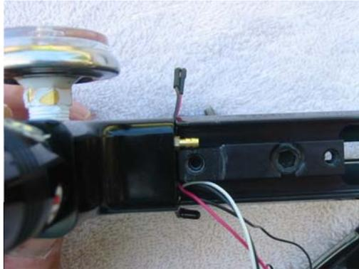
**block**, remove the eyes from the body and make sure eye wires slides easily and that wires are not between the block and the body. Once the wires move easily and the front block is pressed flat against the body tighten the setscrew. **If there is even a small gap between the body and the front block do not tighten. Tightening will crush the eye wire and disable the eye.** Often the eye wires go right into place and this is a very quick and easy step, BUT it can seem
