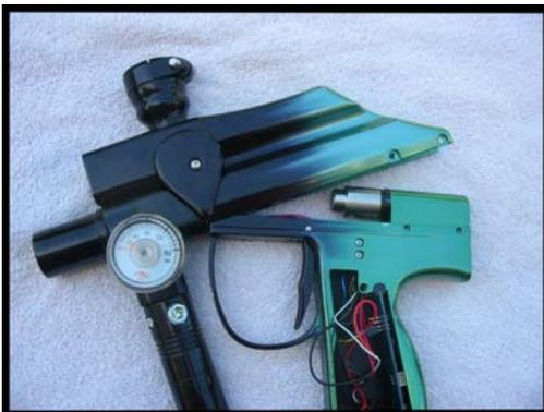
Hinge it apart if it's a bit sticky. It will easily come apart but be careful not to pull on the wires. Wires should easily slide up from trigger housing. Feed the wires up as necessary.
