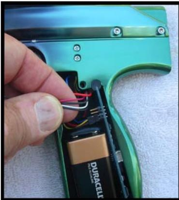
Second, take the four screws off the back of ram and the one off under the trigger guard and gently pull the marker apart making sure the ram stays attached to the trigger frame.
