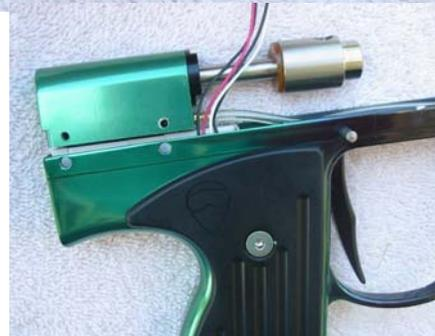
It is best NOT to take the board out of the marker! The alignment of the board in the marker is critical to the proper operation of the On Off switch, the On Off pin is easily lost, and the Equalink port can be broken while sliding the board back into place. No repairs or service is useful by removing board. Should the On Off pin become so dirty as to be unmovable it would be better to remove the wiring harness and wash the trigger frame with the board in place than to remove the board.
