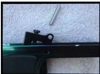
Sixth, you may want to take the pin out and remove the trigger to clean and "lightly" oil it. In the case of a sticky trigger the stop plate does not have to be removed and the ram does not have to be taken out of the grip frame. Push the trigger pin out and clean pin and clean the inside of the trigger with a Q Tip
