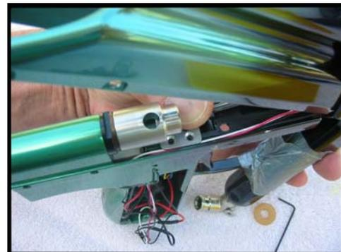
Start screw in front screw of trigger plate. Check that all wires are in groove and tighten, do not over tighten. Slide hammer forward and screw in second screw. Align hammer so the hole is at the top.
