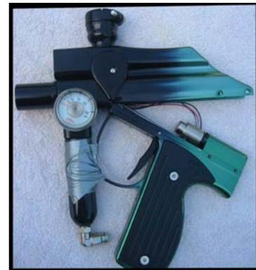
Place the trigger spring back into trigger. Pull excess wires into frame, push hammer back into ram. And route hose into groove next to trigger. Straighten wire along side of trigger frame and into groove next to trigger and opposite hose. Align trigger stop over screw holes in trigger frame and over trigger return spring.
