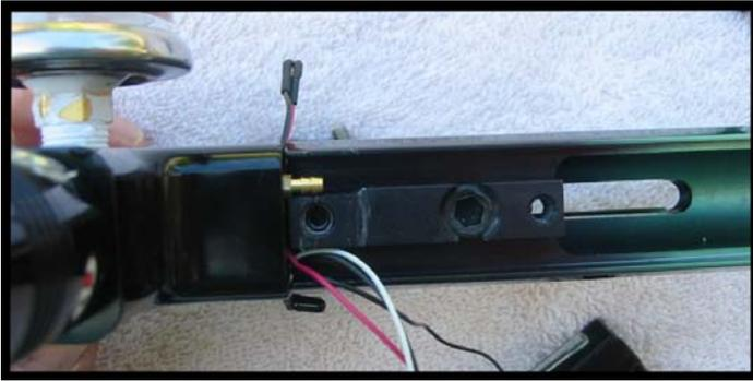
Remove the Front Block; the hose can be left attached to the ram. Place the Valve pin, valve spring and the two setscrews in a small receptacle so they won't get lost.
