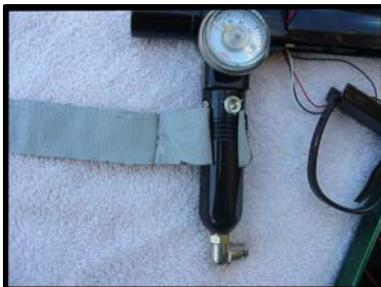
Forth, it is easier if you take a piece of tape and wrap it all the way around the regulator first to avoid scratches. Trigger frame rests inside the body cuts, tape the trigger guard to the regulator.
