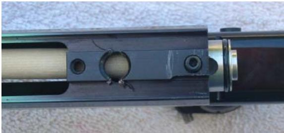
With a wooden dowel, and pushing from the back of the valve towards the front of the marker, push the valve out of the receiver body. The valve's sweep features are now visible, the oval outlet hole and the radius on the valve's back wall.
