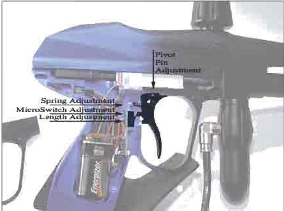
This drawing is for illustration. You may adjust any of the three set screws without removing the clamshell grip frame. However, to adjust the pivot pin, remove the clamshell.
